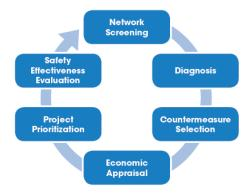
Figure 1. HSM 6-Step Roadway Safety Management Process
