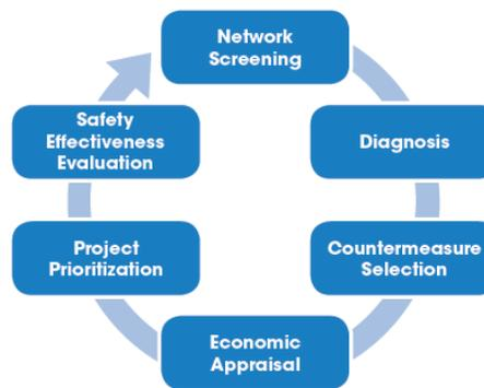
Figure 1. HSM 6-Step Roadway Safety Management Process
